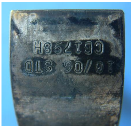
Used bearing shows how heavy stamping disrupts the back contact
