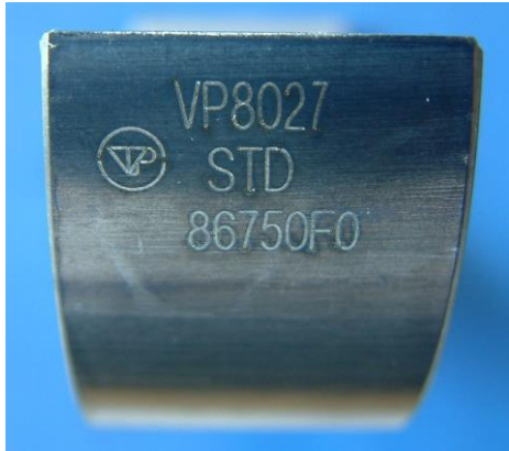
Laser marking on a new bearing (Main bearing for BMW Mini Cooper S 1.6L)
