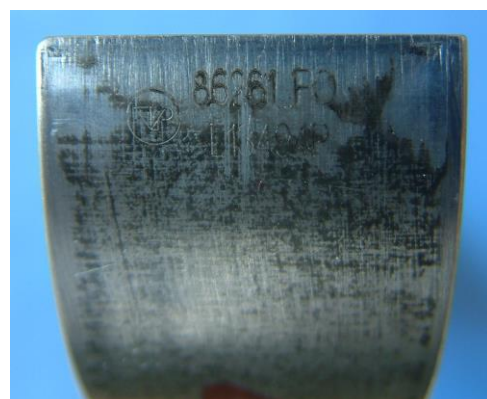
Used bearing shows how laser marking does not interfere with the back contact
